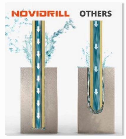
Novidrill 400/500-III third generation models use ordinary tap water as dielectric. This coupled with a high-pressure waterjet air pump system to provide for excellent flush and stability at the electrode during the burn makes the set-up operation more user friendly while keeping work free of oils or other contaminates. It reduces drastically the "bullet nose" effect.
