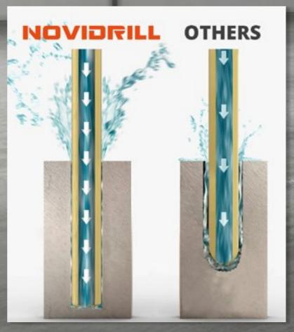
Novidrill third generation models use ordinary tap water as dielectric. This coupled with a high-pressure waterjet air pump system to provide for excellent flush and stability at the electrode during the burn makes the set-up operation more user friendly while keeping work free of oils or other contaminates. It reduces drastically the "bullet nose" effect.
